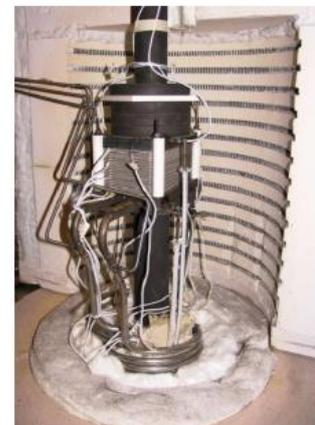
*Elcogen stack being tested for performance at VTT facilities*
